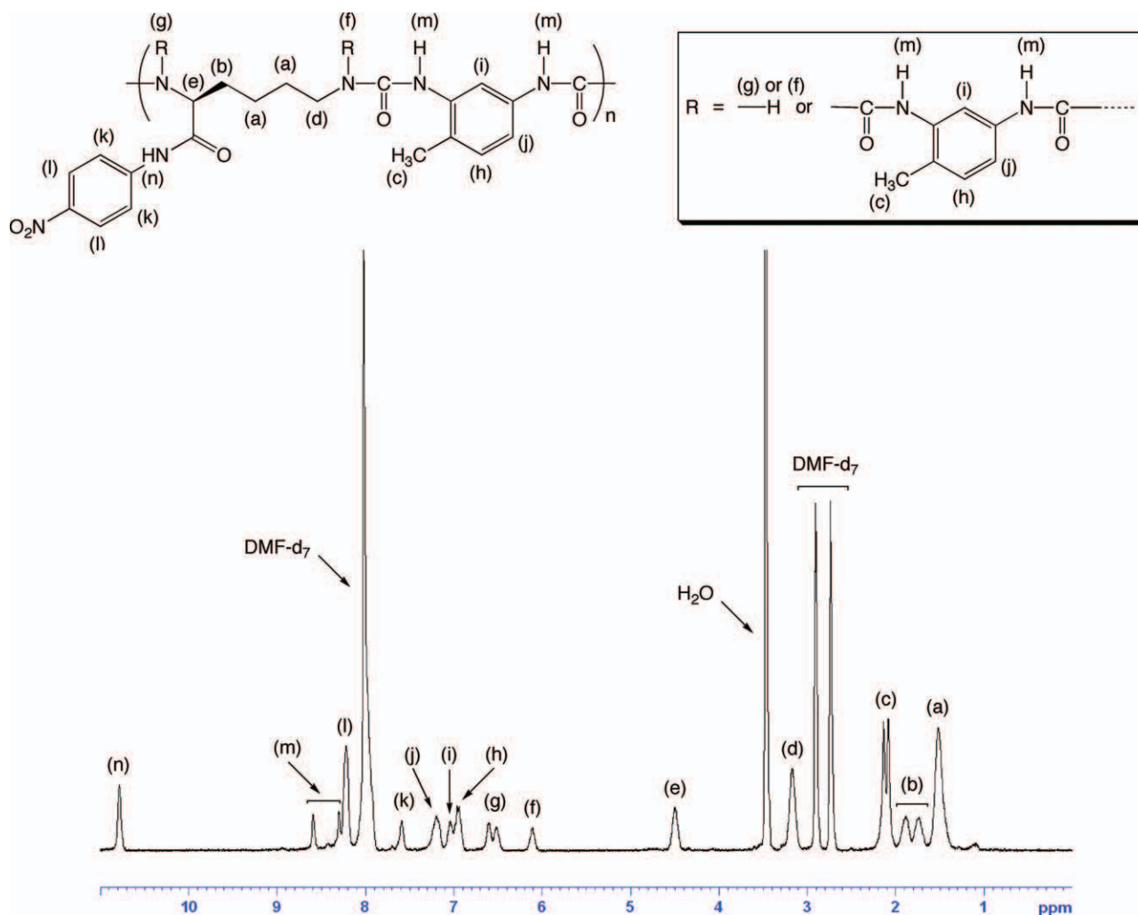
Figure 4. ^1\text{H} NMR spectrum of chiral polyurea (Exp. No. 5 in Table I). (300 MHz, \text{DMF-d}_7 ). [Color figure can be viewed in the online issue, which is available at wileyonlinelibrary.com .]
